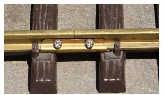
or the inside of code 332 rail (LGB or Aristo); on smaller rail check the flange clearance before installing the screws on the inside of the rail. When possible install both screws on the same side of the rail. Be sure to put a screw in the end of the rail joiner that it is factory attached to the rail. Very often the factory-attached end is the one that will loose electrical contact.
